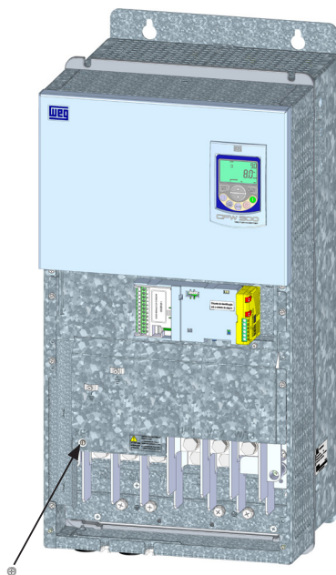
Figure A.4: Location of filter capacitors ground disconnection points - disconnection trough bolts - frame sizes F and G
