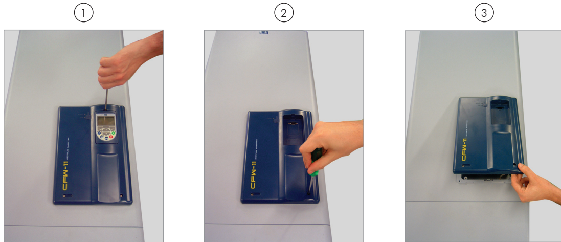
Figure 3.12 - Removal of the HMI and the control rack cover - frame sizes F, G and H
