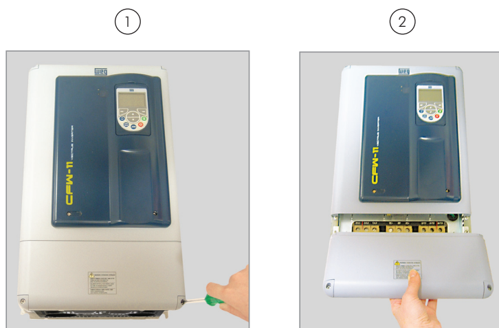
Figure 3.11 - Bottom front cover removal - frame sizes D and E
