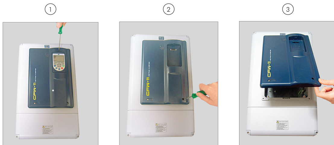
Figure 3.10 - HMI and control rack cover removal - frame sizes D and E
