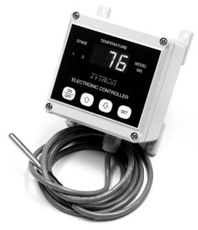
is standard and a 24VAC input is available as a factory option. Two (2) SPDT output relays conservatively rated for up to 10 Amps Resistive and 1/2 HP Motor are provided for each stage. Heavy duty screw terminals with wire clamping plates are provided for all electrical wiring connections. Provision is made for a standard 1/2" electrical conduit connection.
