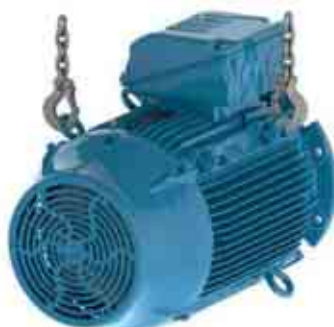
Figure 4.19 - Final result: motor placed in horizontal position
