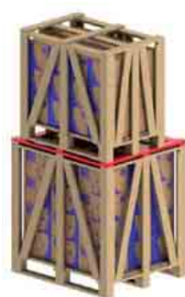
Figure 5.5 - Use of additional battens for stacking
