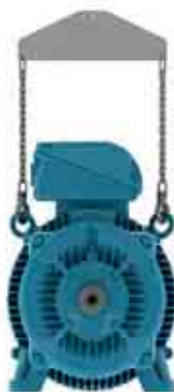
Figure 4.6 - Use of a spreader beam for lifting
