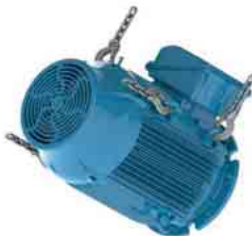
Figure 4.18 - Motor is being rotated to horizontal position
