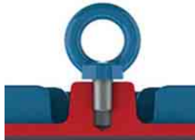
Figure 4.2 - Incorrect tightening of the eyeboll
