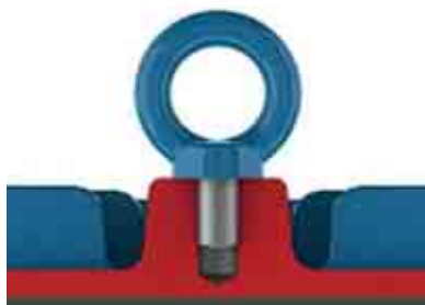
Figure 4.1 - Correct tightening of the eyeboll
