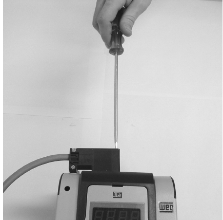
18. Screw on the extern connector Atornillando el conector Parafusando o conector externo
