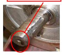
Shaft broken at keyway
