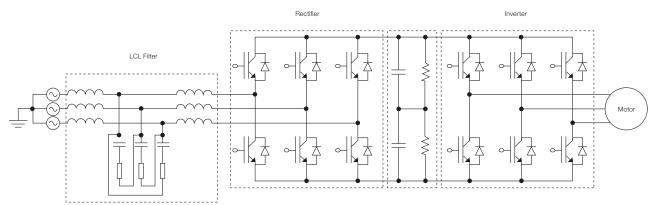
This is an especially attractive solution when it is possible to regenerate power to the grid or when several motors are driven by a single DC link.
