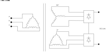
The use of inverters with 12-pulse rectifier complies with the limits recommended by IEEE 519.
