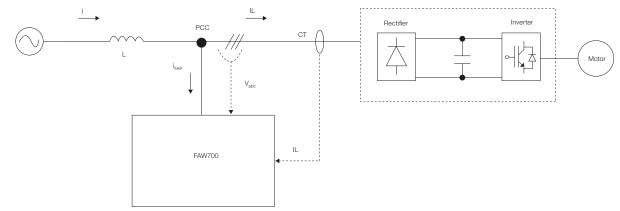
The active filter reduces harmonic currents, improving the system performance. This is a great solution to eliminate harmonics generated by various devices. Because it is relatively new, its cost is higher than the passive filter.
