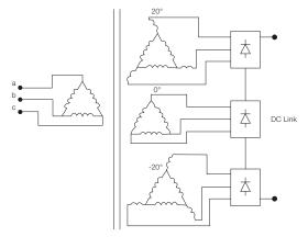
The use of inverters with 18-pulse rectifier complies with the limits recommended by IEEE 519.
