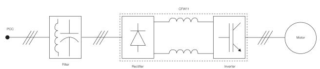
The use of inverters with passive filter at the input complies with the limits recommended by IEEE 519. This is a traditional solution to mitigate harmonics, but it increases heat losses and reduces the power factor.
