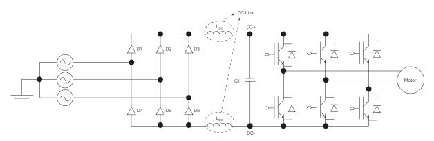
The use of inverters with DC link inductor significantly reduces harmonic emission compared to 6-pulse inverters without inductor in the link.
