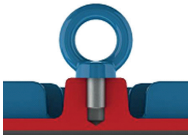
Figure 4.1 - Correct tightening of the eyebolt
