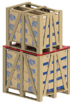
Figure 5.5 - Use of additional battens for stacking
