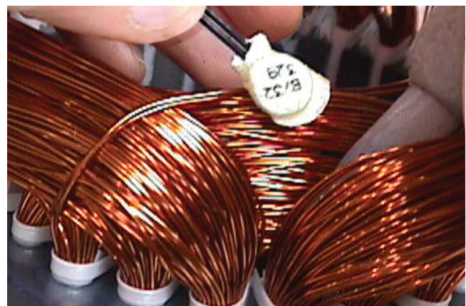
Figure 7.6 - Thermostat installation in the winding
