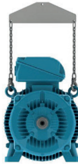
Figure 4.7 - Use of a spreader beam for lifting
