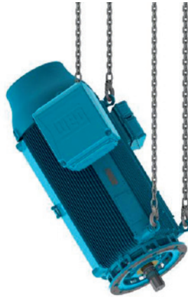
Figure 4.14 - Placing HGF and W50 motors in vertical position
