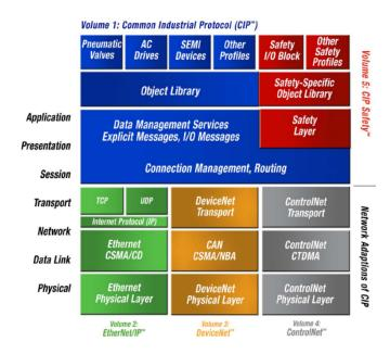
Figure 1.2: CIP protocol structure in layers
