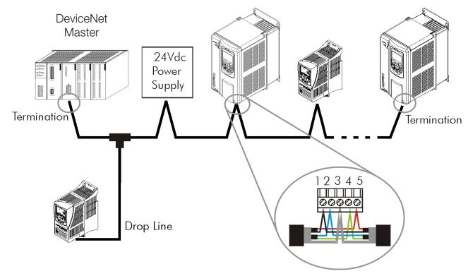
Figure 3.1: DeviceNet network installation example
