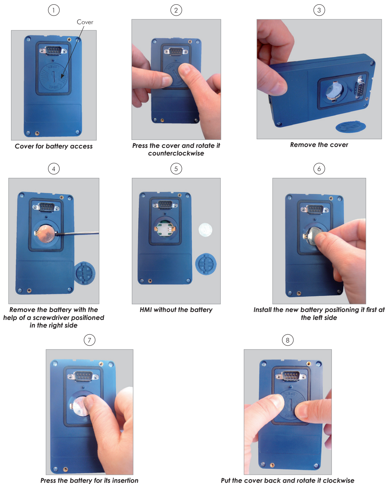
Figure 4.2 - HMI battery replacement
