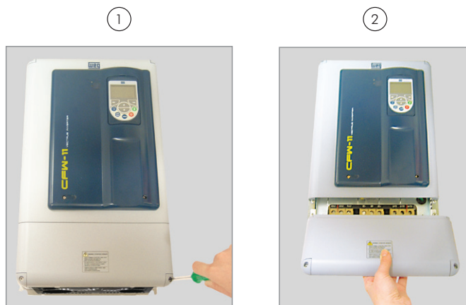
Figure 3.7 - Bottom front cover removal
