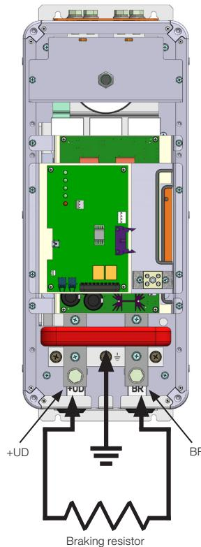
**Figure 3.4:** Connections of the grounding and braking resistor
