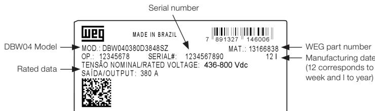
Figure 2.5: Example of identification label of the DBW04
