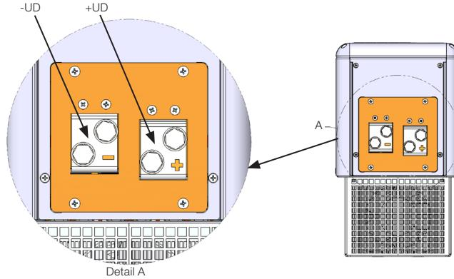
*Figure 3.3: Input connections +UD and -UD*
