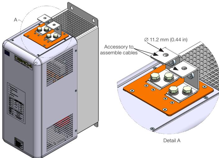
**Figure 3.2:** Accessory for the mounting cables of connections "+UD" and "-UD"
