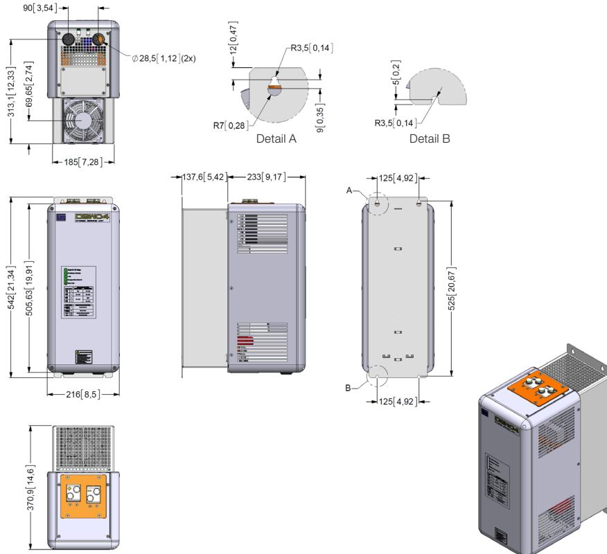
*Figure 7.1: Dimensions of the DBW04 in mm [in]*
