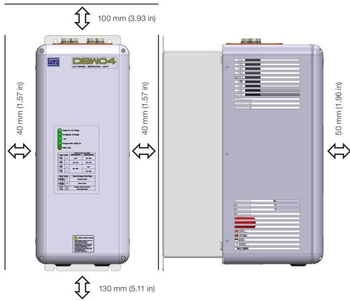
**Figure 3.1:** Free spaces for ventilation
