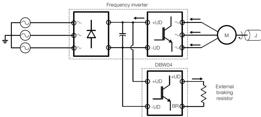
Figure 2.2: Braking step
