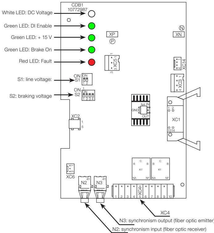
Figure 3.7: Connection points of the CDB1 board
