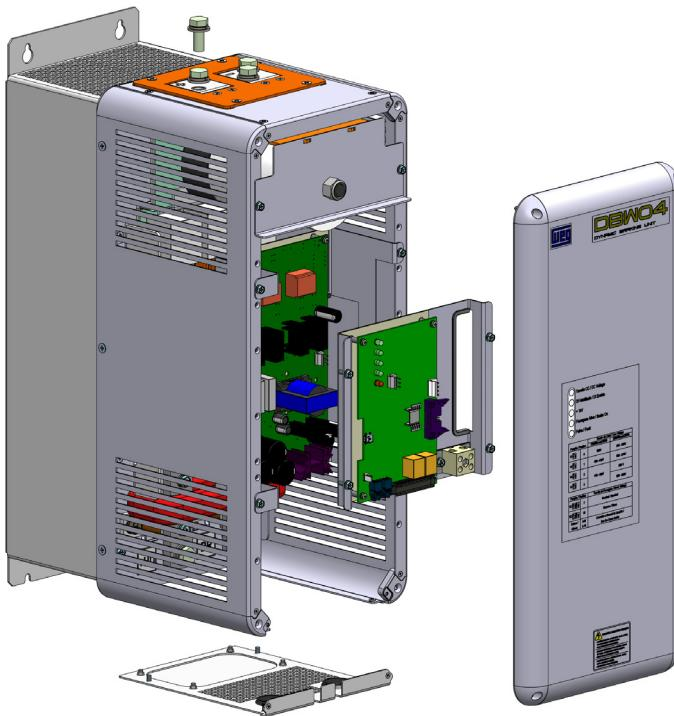
Figure 2.4: Main components of the DBW04 braking module
