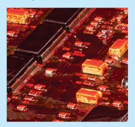
VFD lifespan is extended by a varnish with protection against dust, humidity, high temperatures and some chemicals. This process called **Conformal Coating** (tropicalization) is standard for all CFW, SSW, SCA and MW500 lines, classified as 3C2 according to IEC 60721-3-3.
