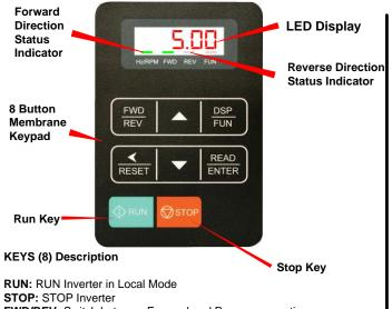
FWD/REV: Switch between Forward and Reverse operation
