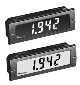
Three power supply choices are available, and a low battery indication is provided for 9VDC battery applications. Mini units feature a standard 3/64 DIN high-impact plastic case. The standard LCD units have a clear viewing window. The units with optional negative image, bright red backlighting, have a red window.
