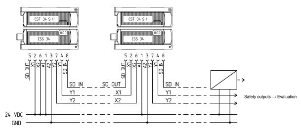
Y1 and Y2 = Safety outputs → Safety monitoring module SD-IN -> SD-i-DP = PROFIBUS
