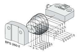
Assured switching distance:  $s_{ao} = 5 \text{ mm}$ assured switch-off distance: sar = 15 mm
