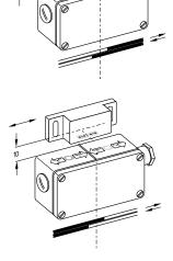
In version -10 and -01: When the switches and actuators come together, the colours must coincide: Red (S) to red (S) and green (N) to green (N).
