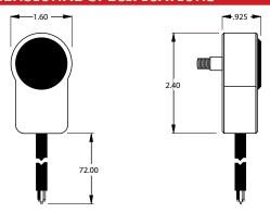
No other mounting brackets or screws are necessary, as the cord will keep the unit from rotating. The PU-E gives a high signal when the south pole of the magnetic disc crosses the Hall-Ef fect transistor. The signal is switched low when the north pole crosses this same transistor.
