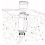
Protected contact block for control devices fitted in switching cabinets with the presence of dust also inside the cabinet. The block ensures an IP67 protection degree for internal electric contacts.
