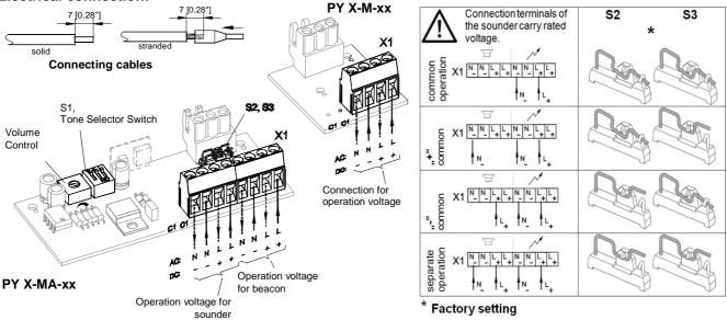
The beacons satisfy the requirements of the standard EN54-23 (Synchronization). **Caution:** In order to ensure synchronization, the devices must be operated with the same potential..
