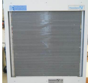
Picture 24 – Condenser external surface
