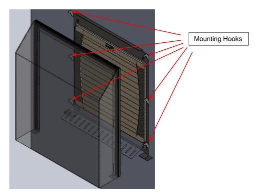
4. Insert wing screw or Allen fasteners through bottom tabs in frame and into the Pemnuts on the tabs of the cover. Tighten fasteners down by hand (standard) or with a 3mm allen key (security). As fasteners are tightened, cover will be pulled down onto the frame and the cover gasket will be compressed against the outer enclosure wall, creating a seal. Tighten until tabs on cover contact tabs on mounting frame (approximately 5 Newton-meters torque).
