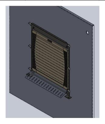
Assembled Frame with Spray Deflector (deflector transparent for clarity)
