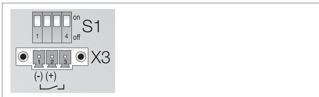
Figure 3.3 X3 terminals and S1 function switches
