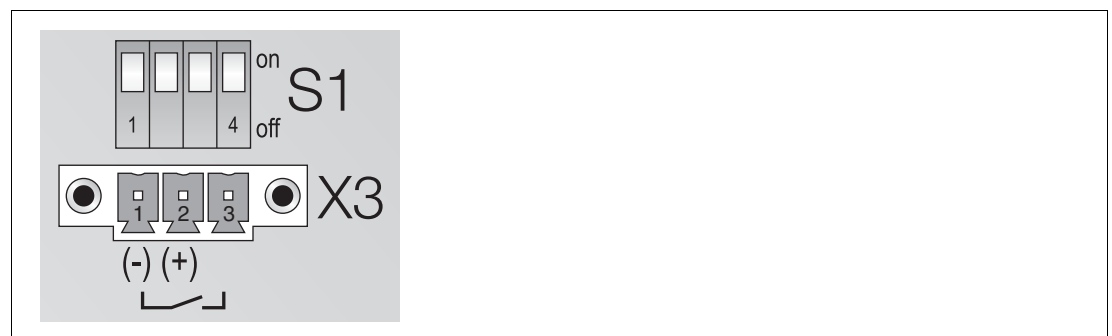
Figure 3.9 X3 terminals and S1 function switches
