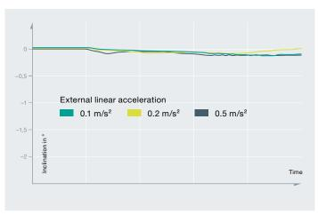
Compensation for external acceleration by F99-Fusion
