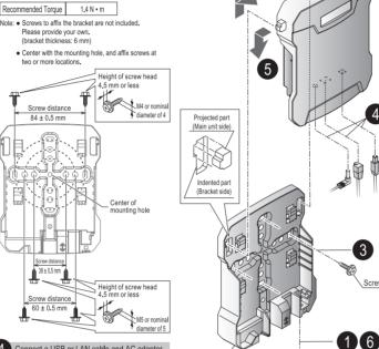
4 Connect a USB or LAN cable and AC adaptor or power terminal to the main unit.
