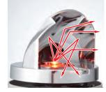
The PATLITE LED revolving warning light uses a unique and patented reflecting system, solely designed for these models. Even though the dispersion characteristics of the LED chip is less than an incandescent bulb, PATLITE's unique design creates an equivalent dispersion effect with the light reflector.
