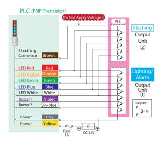
Note: When connecting the PLC outputs for illumination and flashing functions, the wiring (Common Wires) has to be separate between the flashing and non-flashing circuits.
