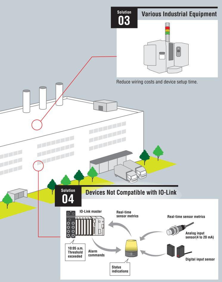
Enables integration of non-compatible devices into IO-Link.
