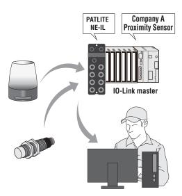
The IO-Link master acquires real-time operational data of the sensors and other devices that are connected. This data can be monitored remotely, and collected for further analysis.
