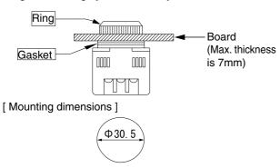
X According to the thickness of the board decrease or increase the gaskets.
