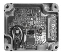
Figure 10 - J4 and J5 position within the transmitter
