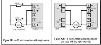
LOAD represents the output signal measurement equipment (controller, register, etc).
