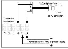
Figure 05 - TxConfig Interface connections - Loop powered
