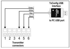
Figure 03 - TxConfig Interface USB connections
