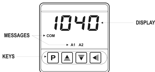
Figure 06 - Identification of the front panel parts
