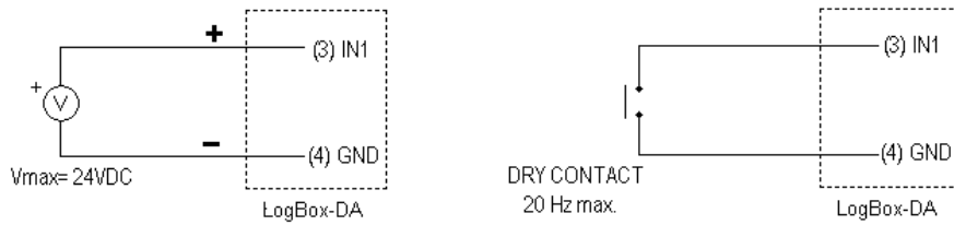
Fig. 10 – Voltage pulse and dry contact channel 1 input
