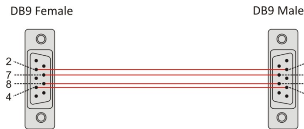
Fig. 26 – Building an extension cable
