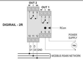
Figure 2 – Electrical Connections
