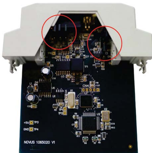
Fig. 5 – Localization of the jumpers in the device
