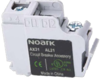
Alarm Switch (AL)/ Auxiliary Contact (AX) (D80)
