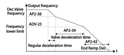
The time set at AP2-39 refers to the absolute time that it takes for the pump to decelerate from the frequency set at AP2-38 to the frequency limit set at ADV-25.
