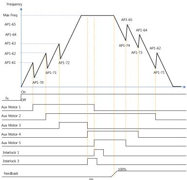
Interlock operation(Op time Order) when Operable Motor and Standby Motor are set to 3 and 2 each
