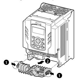
3 Connect the cables to the power terminals and the control terminals. For cable specifications, refer to <u>1.5 Cable Selection</u> on page <u>10</u>.
