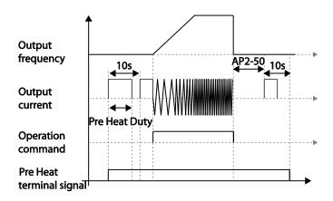
The diagram above shows the operation waveform related to AP2-50 DC Inj Delay T. The Pre Heat function performs when the inverter stop mode is set to Free Run and the Pre Heat signal is supplied. Then, if the inverter operation command is on, the inverter maintains acceleration and a fixed frequency. If the inverter operation command is off, the motor is in Free Run and the Pre Heat operations starts after the time amount set in AP2-50.
