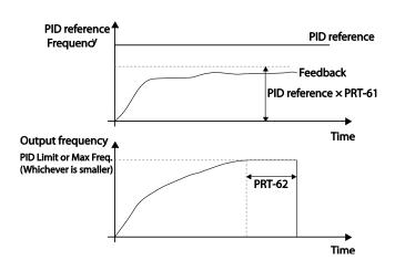
In the graph above, Pipe Break occurs if the feedback is smaller than the value caculated by multiplying the two values set at PID-04 and PRT-61(PID-04 x PRT-61) at the inverter's maximum output (when PID output is the maximum set value, or the inverter is running at the frequency set at DRV-20).
