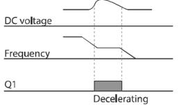
PRT-51 Stall Freq 1– PRT-58 Additional stall protection levels can be configured for different frequencies, based on the load type. As shown in the graph below, the stall level can be set above the base frequency. The lower and upper limits are set using numbers that
