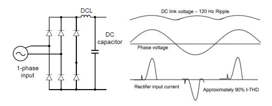
Figure-2 Typical Single-Phase Configuration
