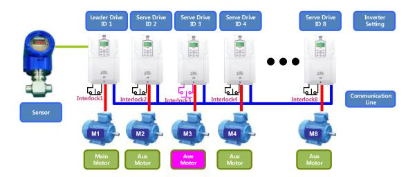
The picture below shows the function in case that M3 becomes HAND/OFF State or interlock and Trip are caused.(supposing that the priority is not changed),(interlock is the function corresponding to B terminal(Normal close)).
