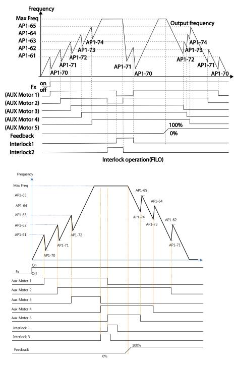
Interlock operation(Op time Order) when Operable Motor and Standby Motor are set to 3 and 2 each
