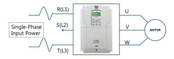
Figure-3 Terminal Wiring Diagram
