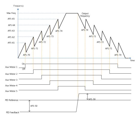
The following diagram describes the MMC basic sequence based on FILO and FIFO settings.
