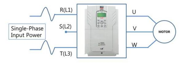
Figure-3 Terminal Wiring Diagram
