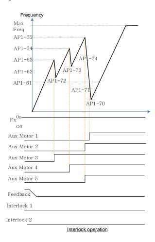
In case that Operable Motor and Standby Motor are set to 3 and 2 each, it operates in the order of "Aux Motor 2  $\leftarrow$   $\rightarrow$  Aux Motor 4  $\leftarrow$   $\rightarrow$  Aux Motor 5".
