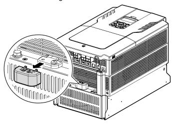
2 Remove the EMC ground cable from the right terminal (EMC filter-ON / factory default), and connect it to the left terminal (EMC filter-OFF / for power sources with asymmetrical grounding).
