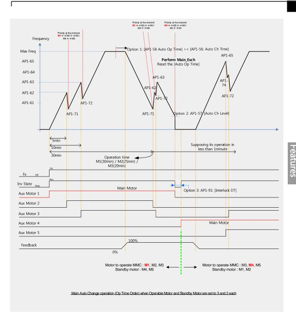
When there is motor trouble, the interlock feature is used to stop the affected motor and replace it with another that is not currently operating (off state). To activate the interlock feature, connect the cables for abnormal motor signal to the inverter input terminal and configure the terminals as interlock 1–5 inputs. Then, the inverter decides the motor's
