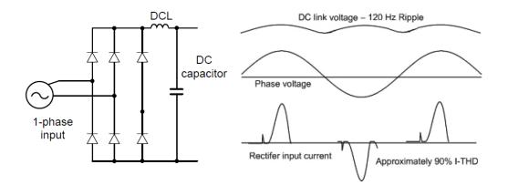
Figure-2 Typical Single-Phase Configuration
