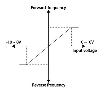
[Bipolar input voltage and output frequency]
