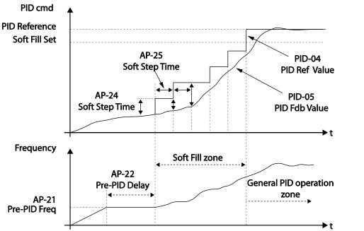
When a PID process is performed after the soft fill PID operation, the PID Reference value becomes the PID-11 PID Ref1 Set value.
