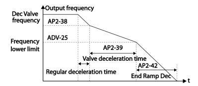
The time set at AP2-39 refers to the absolute time that it takes for the pump to decelerate from the frequency set at AP2-38 to the frequency limit set at ADV-25.
