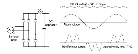
Figure-1 Typical Three-Phase Configuration
