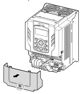
2 Push and hold the levers on both sides of the cable guide (①) and then remove the cable guide by pulling it directly away from the front of the inverter (②). In some models where the cable guide is secured by a bolt, remove the bolt first.
