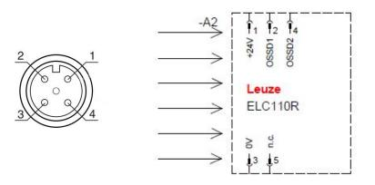
Fig. 6.2: Pin assignment and connection diagram receiver
