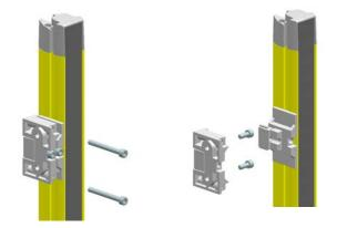
Fig. 5.7: Mounting via swiveling mounting brackets BT-2SB05 and M5 screws
