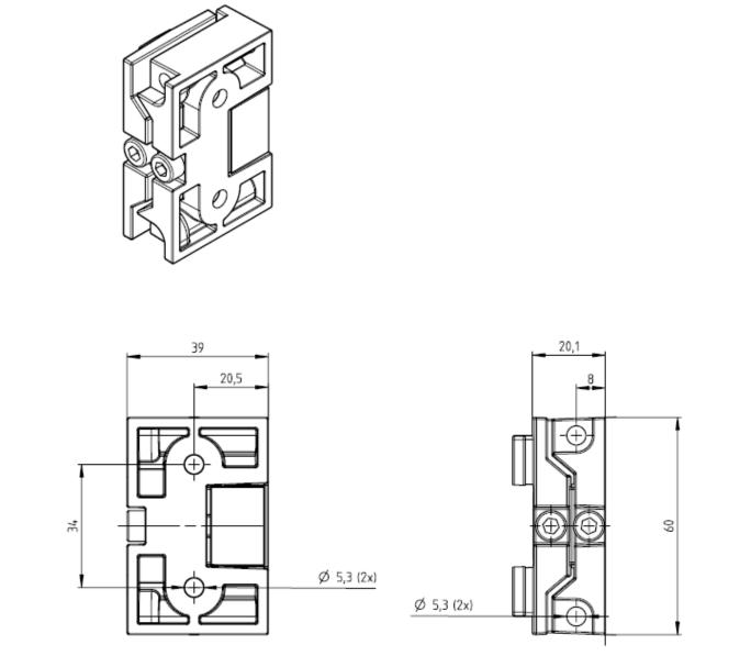
Fig. 12.2: Swiveling mounting bracket for groove mounting BT-SB05
