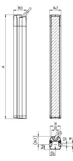
Fig. 12.1: Dimensions of transmitter and receiver
