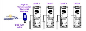
Note that the gateway needs an external 24Vdc, 300mA power supply. This is not shown in the above diagram. The gateway is supplied with a RJ11 to D-type connector, which will connect to the first drive. For each additional drive in the network, a RJ11 splitter and a RJ11 data cable are required (available from your Optidrive supplier).
