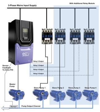
Relay 1 on the standard I/O terminals of the Drive (T14 & T15) cannot be used as part of the DOL control but is freely programmable to other functions through parameter P2-15. Relay 2 on the standard I/O terminals of the Drive (T17 & T18) can be used as the DOL control for the first slave pump. Relay 2 is set to DOL control by setting parameter P2-18 = 8, or can be used for an alternative function by setting a value other than 8.
