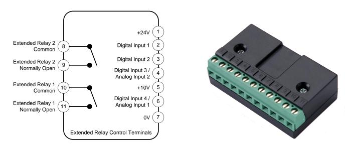
The Option module is fitted to pins 1 - 11 on the drive control terminal block of the Optidrive E2.
