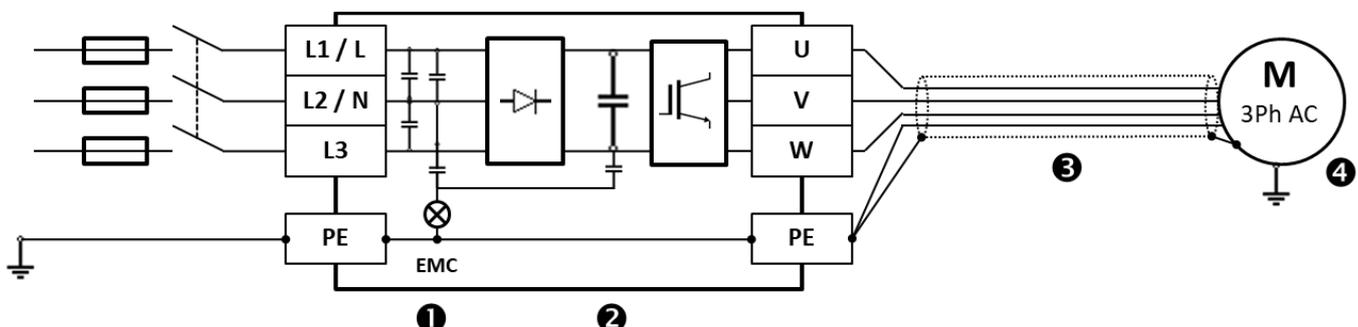
During normal operation, leakage currents may be present at the points indicated. These are:
