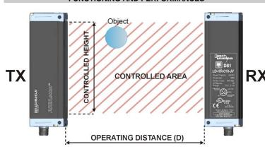
The beam interruption due to the passage of an object inside the controlled area caused the closing of the switching output and the variation of the device analogue output signal. Small objects can be detected (reaching dimensions of only 5 mm) and determine linear measurements with a +3 mm error in best cases.
