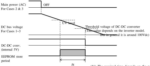
(\*1) The required time depends on the parameters Around 0.5~1s or more which have changed before power OFF.
