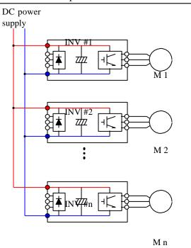
Case 2: Connected in parallel to an AC-fed inverter
