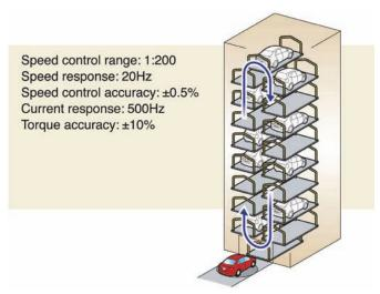
Figure 3. Sensorless Vector Control
