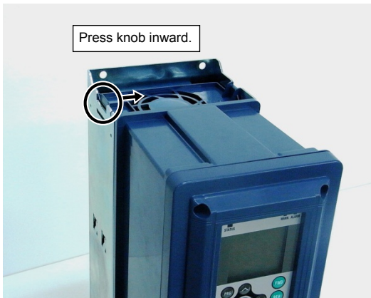
Remove the cooling fan (with case).
