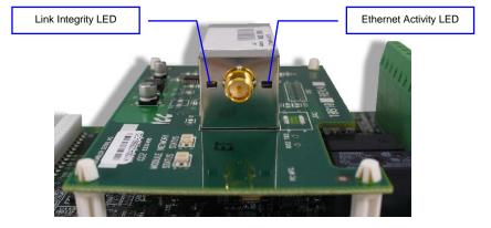
Figure 4: Wireless Network LED Indicators
