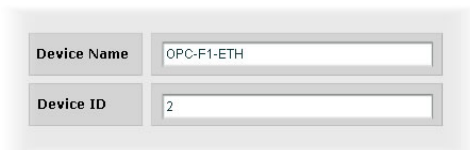
Figure 24: BACnet Device Identifiers
