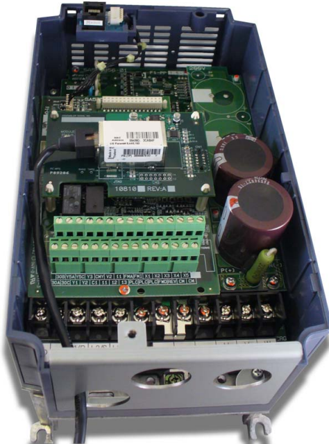
Figure 6: Example Ethernet Cable Routing
